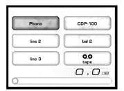
The **operational menu** provides easy access to the most basic functions of the preamplifier: **input selection** and **tape monitor**. It also provides both a numeric and a graphic depiction of the current **volume** setting.
